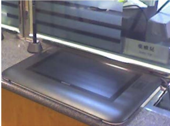
*Wacom interactive pen displays combine the benefits of an LCD monitor with Wacom's patented pressure-sensitive pen input to control the cursor and capture electronic handwritten signatures.*
